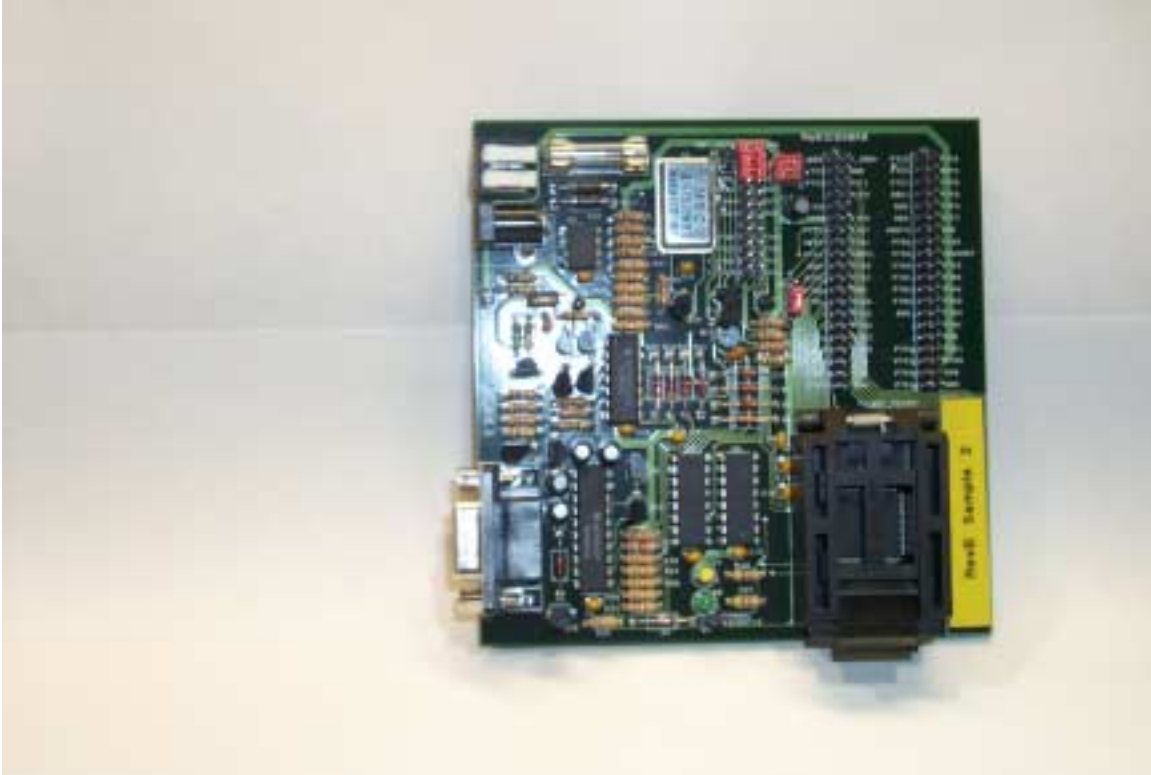
Figure 1-1 M68ICS08AB ABICS In-circuit Simulator Board
